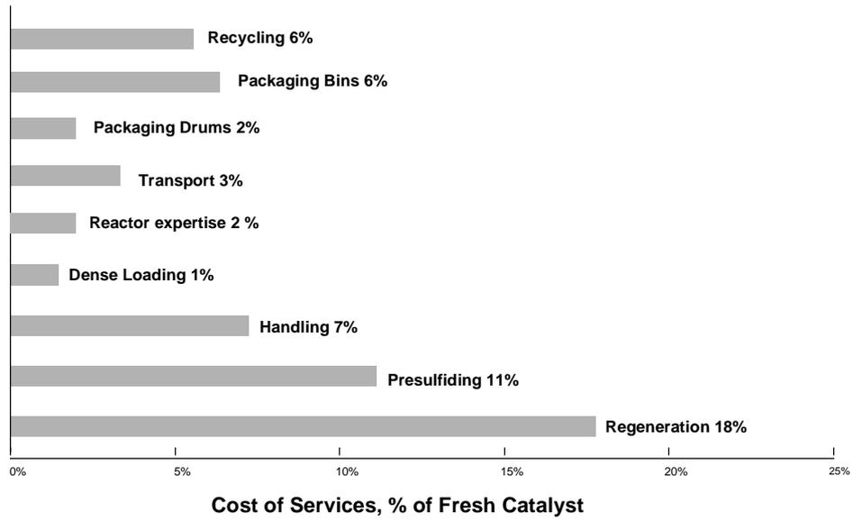
*Figure 7 : Cost of off-site services vs fresh catalyst*
