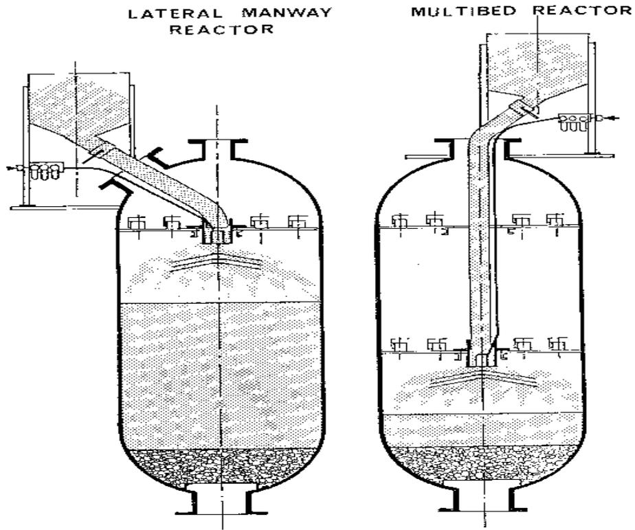
*Figure 5 : Application of Densicat to particular reactor types*
